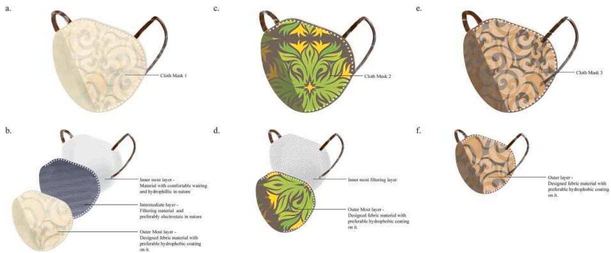
Fig. 3. Diagram shows the different types of cloth masks and their layering pattern: a. Cloth Mask 1 b. Different layering pattern of Cloth Mask 1 c. Cloth Mask 2 d. Different layering pattern of Cloth Mask 2 e. Cloth Mask 3 f. Different layering pattern of Cloth Mask 3.
